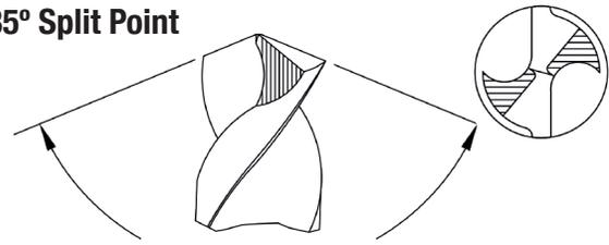
Drill Harder Steel Alloys - Self-Centering
