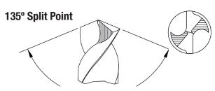
Drill Harder Steel Alloys - Self-Centering Ideal For Use In Handheld Power Drill Requires Less Operator Force Than 118° Point Drills
