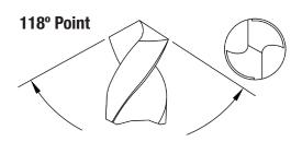
General Purpose Use - Not Self-Centering Ideal For Use In Stationary Drill Press For Drilling Softer Materials Like Wood, Aluminum And Low To Medium Steel Alloys
